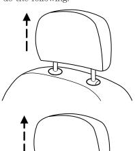
2. Simultaneously press and hold both the adjust/release button and the unlock/remove button, then pull up on the head restraint.
